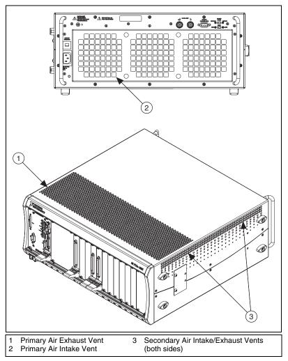
Figure 2-2. NI PXIe-1065 Vents
